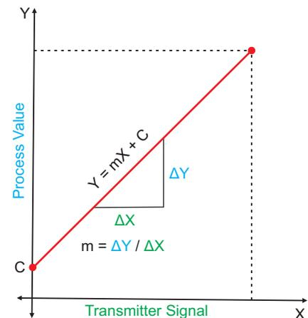
As is evident from the aforementioned transmitter examples, different transmitters produce signals varying both in type (mV/V/mA) and range. Most PPI instruments, thus, provide programmable Signal Type and Range to facilitate interface with a variety of transmitters. A few industry standard signal types and ranges offered by the PPI instruments are:  $\pm 80\text{mV}$ ,  $\pm 5\text{ V}$ ,  $\pm 1$  to  $\pm 5\text{ V}$ ,  $0\text{-}20\text{ mA}$ ,  $4\text{-}20\text{ mA}$ , etc.
