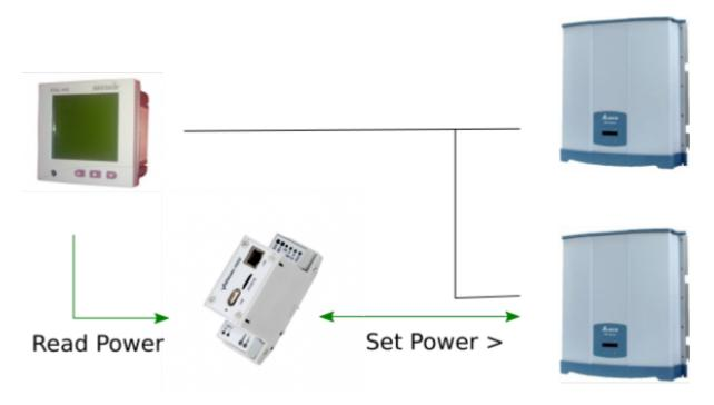
Power control signifies dynamically changing an Inverter's output power based on an algorithm. Wattmon supports dynamic power control using an add-on software package and can be used in conjunction with a power meter for various purposes:
