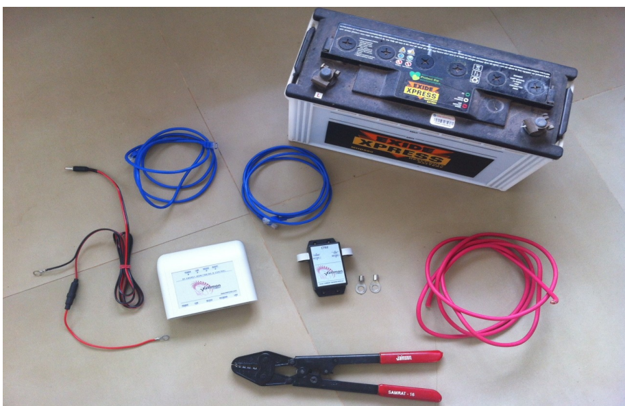
Figure 1.1 Wattmon solar monitoring components prior to hooking up with the battery
