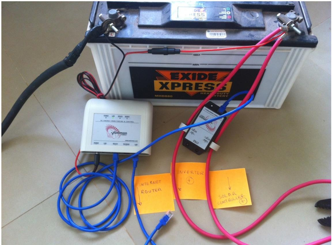
Figure 1.6 Final setup of your WattmonSolar hardware
