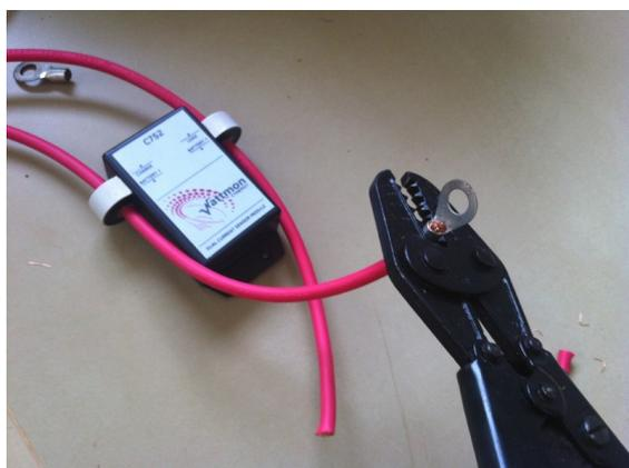
Next, strip the ends of both cables, insert the lugs, and crimp it with a crimping tool or a pair of strong pliers.
