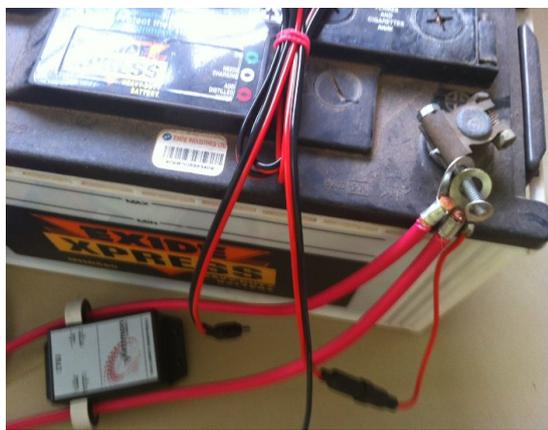
Next, connect both of the thick cables together with the red end of the wattmon power cable to the positive terminal of the battery, and tighten.
